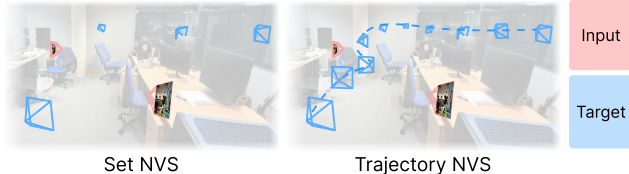
Figure 3. Set NVS versus trajectory NVS. Set NVS generates target views as an image set, whereas trajectory NVS produces them as a trajectory video.
